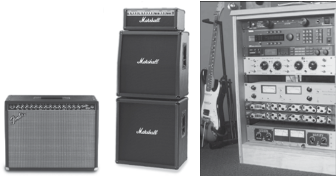
FIGURE 14-7: Amp configurations (from left to right): combo, head and cab/stack, and rack system.
