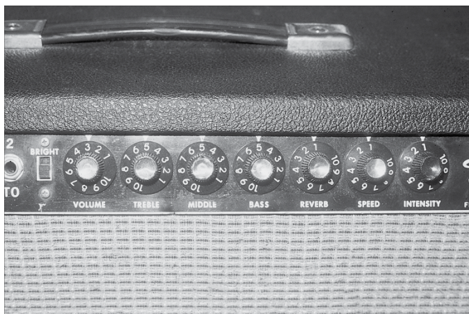
FIGURE 3-9: When starting to build a sound from scratch, place the controls in a neutral position with the volume reduced, the effects off, and the tone controls “flat.”
