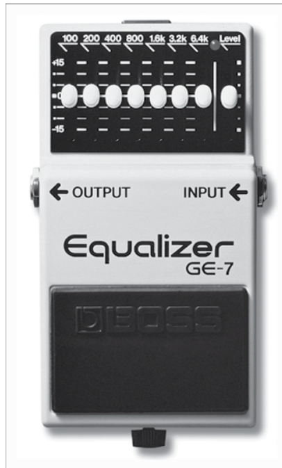
FIGURE 15-4: The Boss GE-7 EQ is a seven-band graphic EQ that covers the core of the guitar's frequency spectrum.
