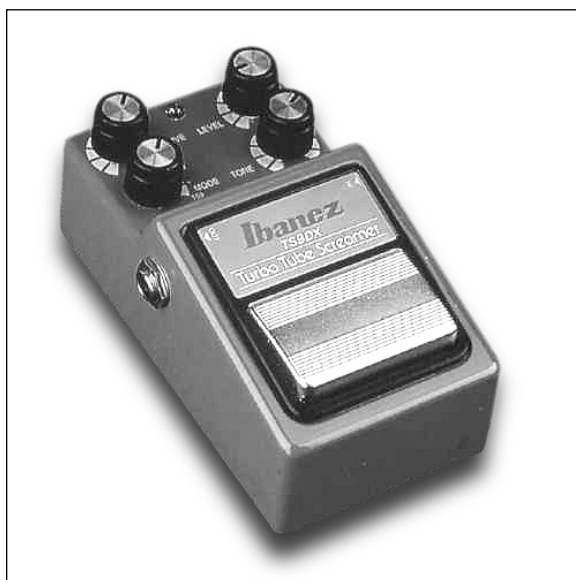
FIGURE 15-1: Although its circuitry is solid-state, the Ibanez Tube Screamer is a classic effect known for its smooth, tube-like overdrive.
