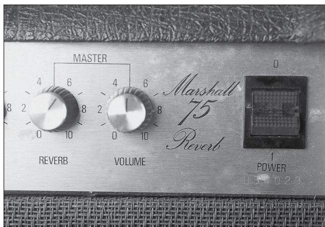
FIGURE 3-5: The control for amp reverb is usually limited to one knob: the volume or intensity of the effect.
