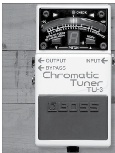
FIGURE 2-7: This Boss TU-3 tuner has a large meter for easy reading of a pitch's flat or sharp status, plus LEDs that show what pitch you're closest to.
