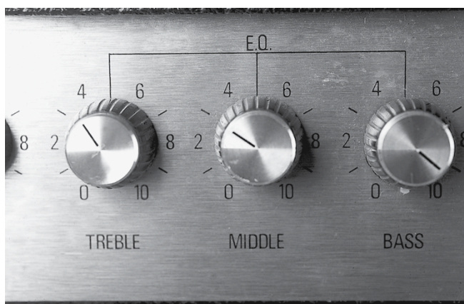
FIGURE 3-4: The tone controls of an amp's EQ, or tone-shaping, section.
