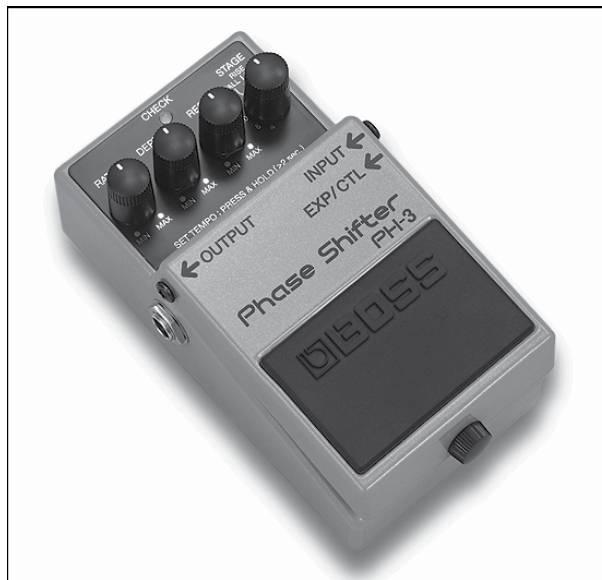
FIGURE 15-7: The phase shifter, like the Boss PH-3 shown here, was a mainstay effect of 1970s rock and has made a comeback in recent years.
