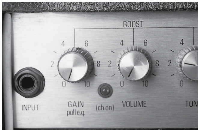
FIGURE 3-3: The tale of two volumes: preamp and power amp, channel and master.
