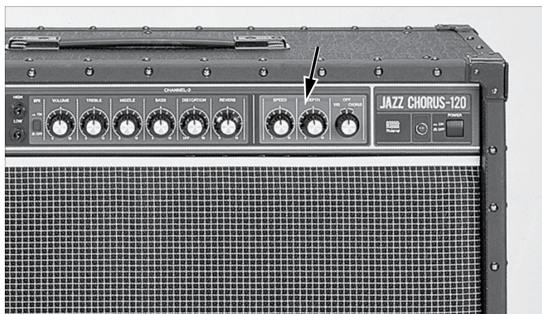
FIGURE 3-6: The two controls that modify the chorus effect on the Roland JC-120 are speed and depth .
