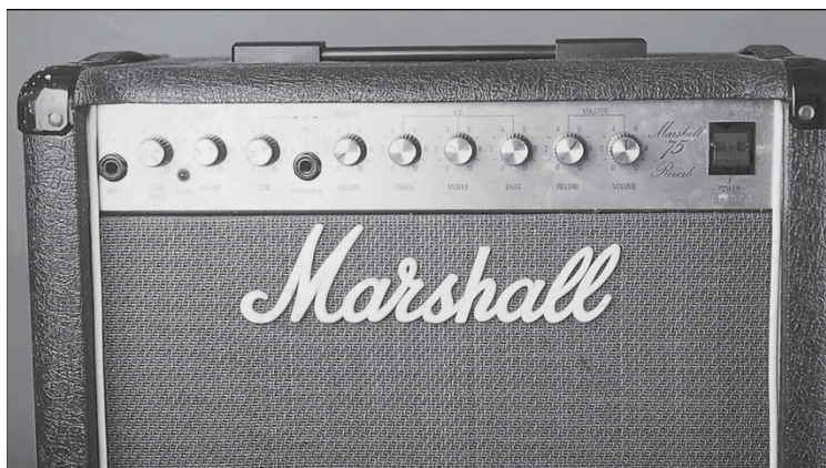
FIGURE 3-2: The control panel groups together and supports the jacks, switches, and knobs of an amp.
