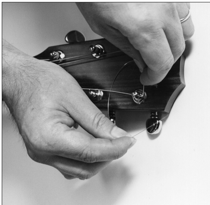
FIGURE 18-2: String kinked to the inside of the headstock, with slack for winding.
