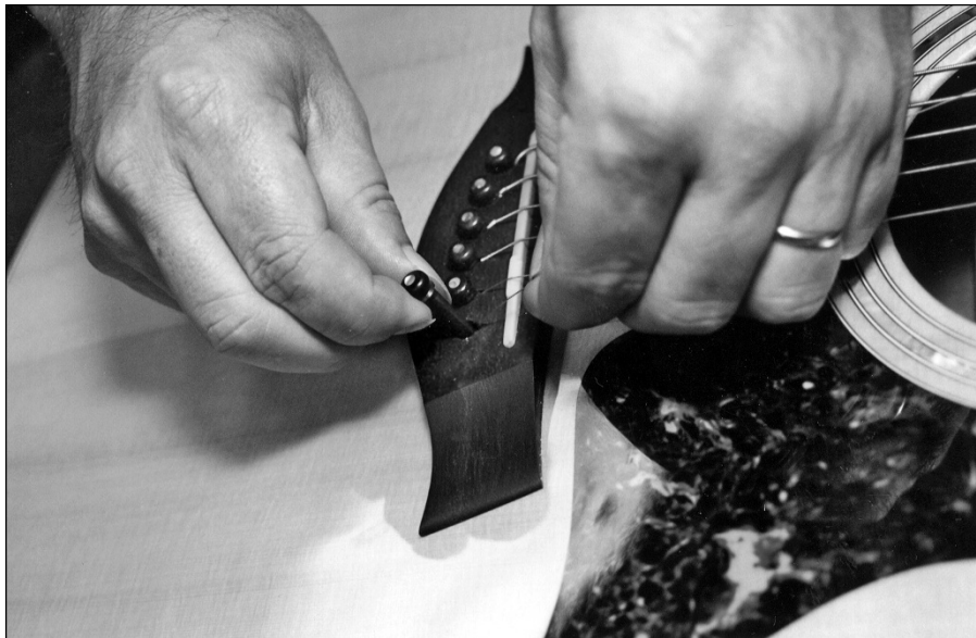
FIGURE 18-1: How to place the new string in the bridge and position the bridge pin.
