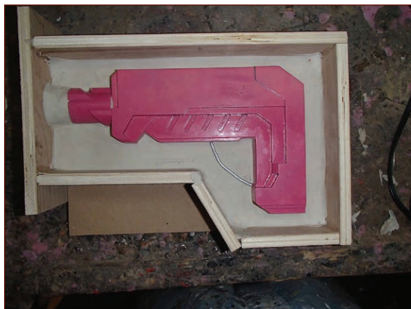
FIGURE 7-6: Sprues will allow the casting material in, while vents will let the air out.
