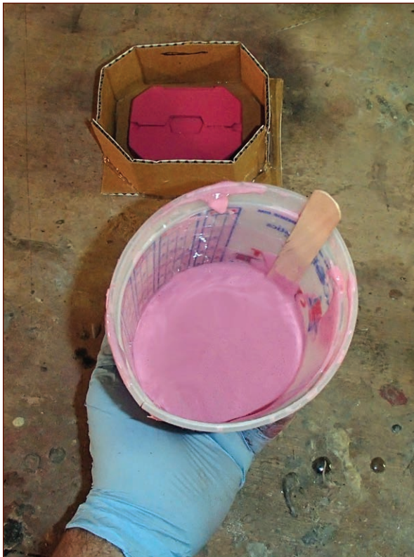
FIGURE 6-5: Properly mixed silicone is all one uniform color.
