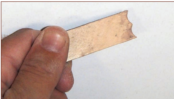
FIGURE 2-52: A contour gauge made by whittling the end of a mixing stick
