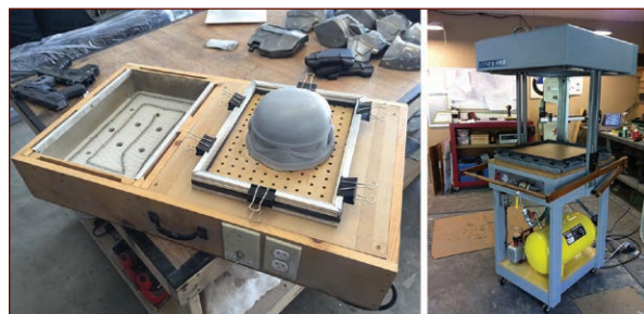
FIGURE 10-34: A Hobby Vac machine built by Liz Hydra of Hydra-works and a customized Proto-former built by Harrison Krix of Volpin Props, both based on plans from build-stuff.com
