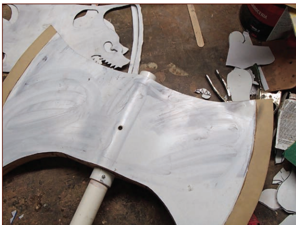
FIGURE 1-38: The handle installed with a set screw
