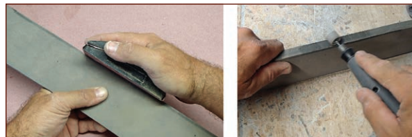
FIGURE 3-4: Smoothing the edges with a sanding block (left) or the rotary sanding drum (right)
