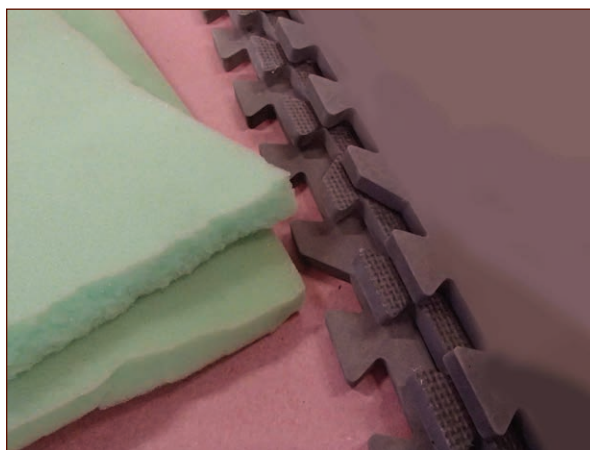
FIGURE 14-2: EVA Foam (right) and upholstery foam (left) are easy to find and easy to use.
