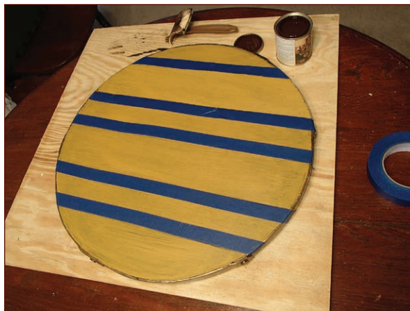
FIGURE 12-18: Masking on the edges of every other plank
