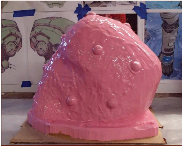
FIGURE 8-14: Silicone registration keys stuck into the tacky silicone surface.
