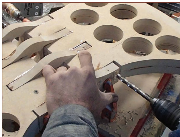
FIGURE 1-27: Making a bigger hole for the screw head to hide in is called "countersinking."
