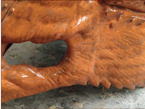
FIGURE 13-31: The basecoat in terra-cotta, all blotchy and uneven
