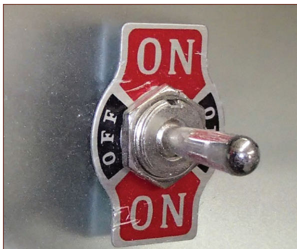
FIGURE 10-31: The toggle switch to select between turning on the heater and turning on the vacuum
