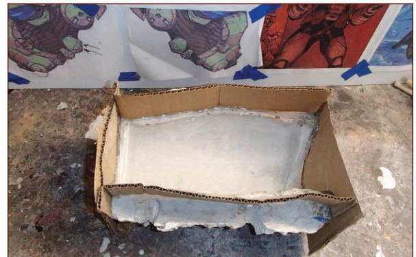
FIGURE 9-14: The open end of the molds closed up with corrugated cardboard and hot glue
