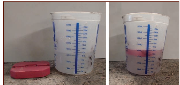
FIGURE 6-11: Using the prototype and a measuring cup to determine casting resin volume
