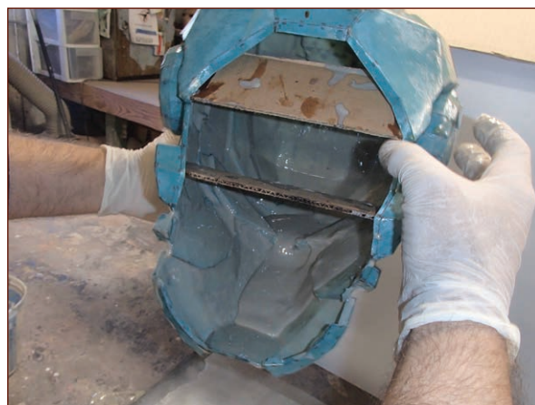
FIGURE 2-43: Keep moving the whole thing in order to keep goop from pooling in one place.
