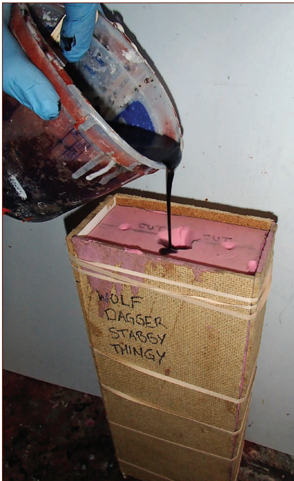
FIGURE 6-37: Pouring slowly and carefully in order to avoid bubbles
