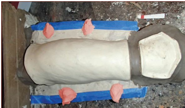
FIGURE 9-12: Clay tabs added to the parting wall will provide starting points when it comes time to pry the two pieces apart.
