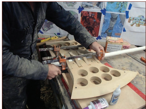
FIGURE 1-24: These are bar clamps, just one of the countless varieties of clamps that you will need more of.
