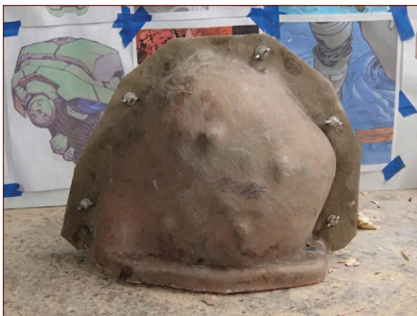
FIGURE 8-36: The reassembled mold; ready to roll
