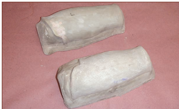
FIGURE 9-17: The finished forming buck after sanding it smooth
