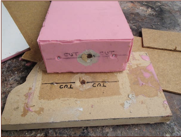
FIGURE 6-30: The ink that was on the inside of the box is now on the outside of the rubber. Sorcery!
