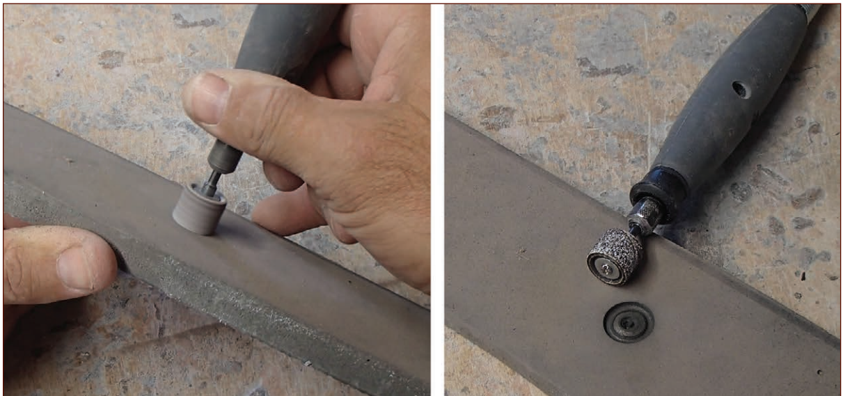
FIGURE 3-57: Simulating a rivet head with the tip of a sanding drum on a rotary tool
