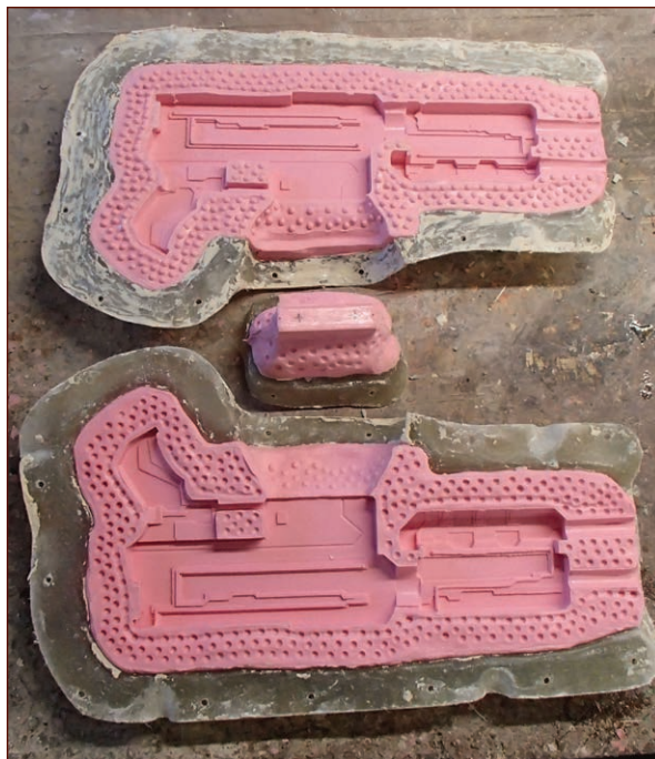
FIGURE 7-58: Rubber jacket halves fitted into mother mold halves
