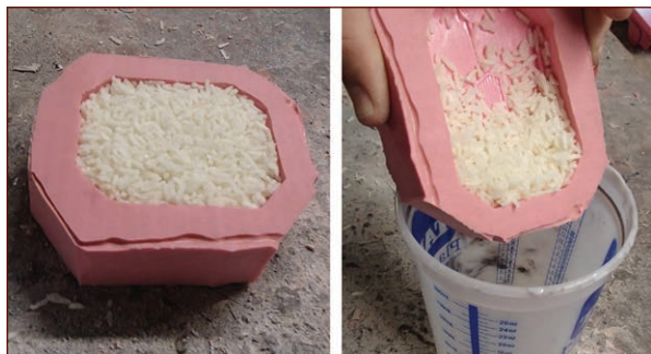
FIGURE 6-12: Using rice to determine casting resin volume
