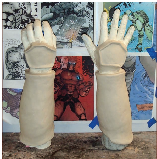
FIGURE 9-6: There's no easy way to get this forearm armor formed in one piece without the plastic sheet locking onto the forming buck.
