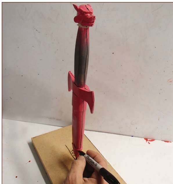
FIGURE 6-23: Marking the sides of the prototype and the bottom of the mold box where the mold will be cut
