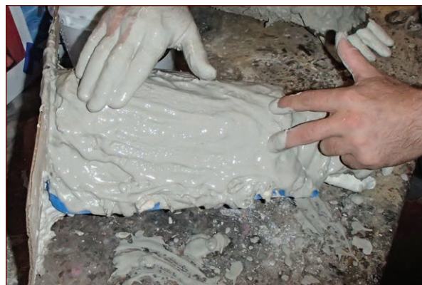
FIGURE 9-9: Thickening the mold with more plaster
