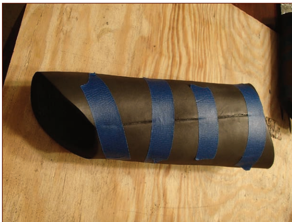
FIGURE 3-40: Masking tape to hold the seam while the glue dries
