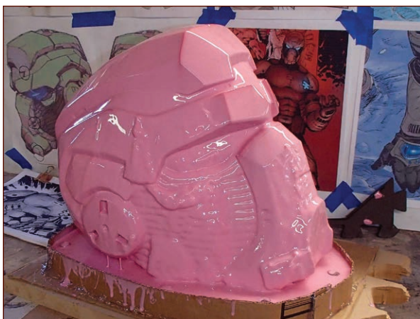
FIGURE 8-12: The cured print coat is thinner in high areas where the liquid rubber flowed away.
