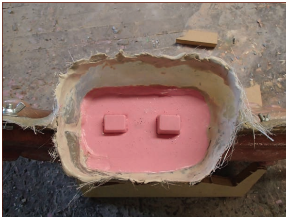
FIGURE 7-54: The hole filled with more rubber, but not completely filled
