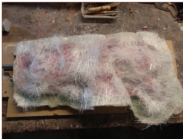
FIGURE 7-37: Fiberglass mat laid evenly over the wet resin
