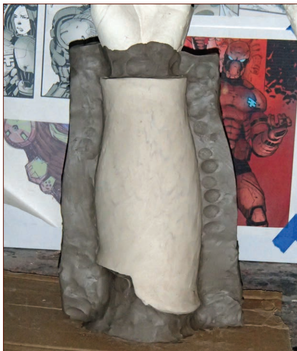
FIGURE 9-7: A parting wall made of water-based clay
