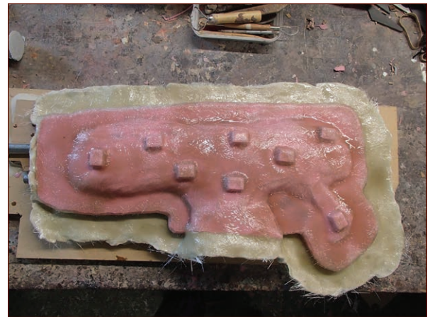
FIGURE 7-39: The first half of the mother mold completed
