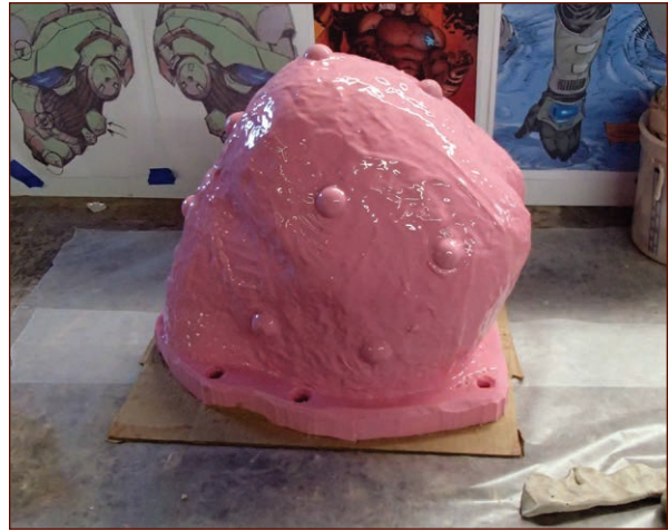
FIGURE 8-15: Pegs and drip wall removed from the bottom of the jacket mold
