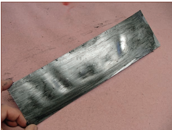
FIGURE 12-7: A decent-looking piece of brushed metal, but made out of plastic
