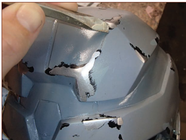
FIGURE 13-24: Adding more scratches to the edges of the masked areas
