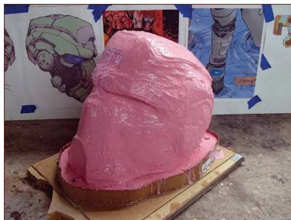
FIGURE 8-13: Thixotropic additive makes this stage a bit like frosting a cake.
