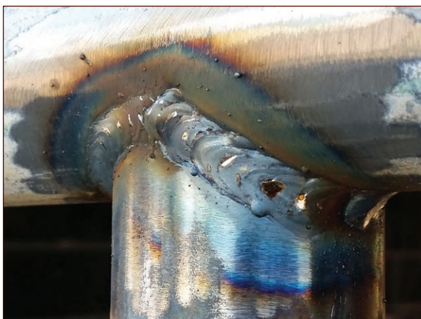
FIGURE 13-51: The heat from welding these two pieces of steel together causes a rainbow of tempering along the edges of the seams.
