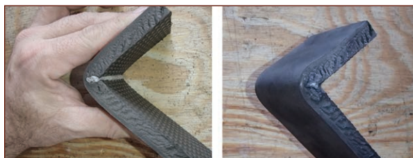
FIGURE 3-11: After gluing the inside corner, the outside is left with a nicely rounded edge.
