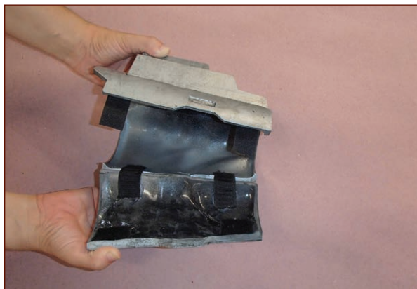
FIGURE 14-13: A gauntlet split along a visible seam with elastic and Velcro installed
