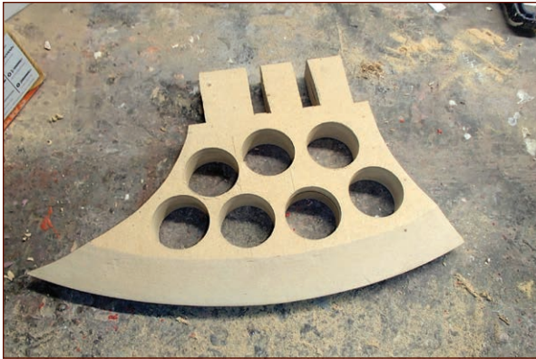
FIGURE 1-21: The hole saw quickly makes Swiss cheese out of the MDF axe blade.
