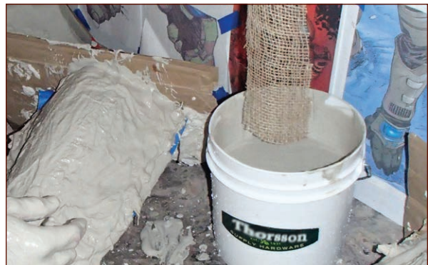
FIGURE 9-11: Plaster-soaked strips of burlap laid into the still-wet plaster will make for a stronger mold.
