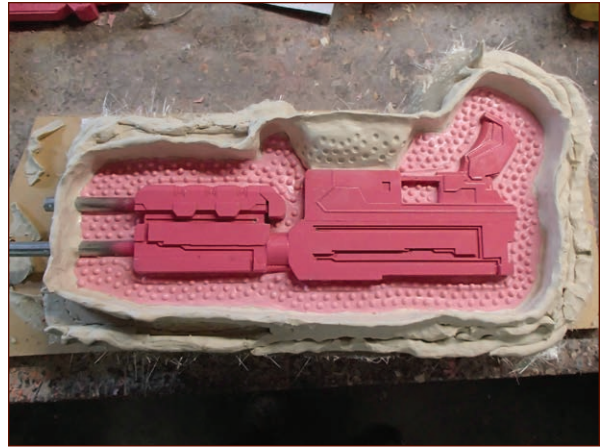
FIGURE 7-41: New drip walls built up on the mother mold
