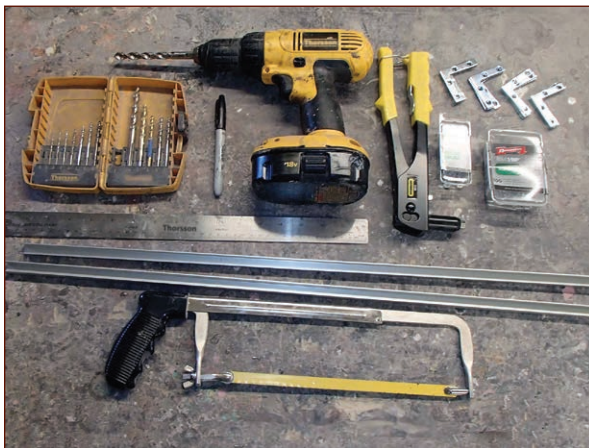
FIGURE 10-1: A drill with a 1/8" bit, a ruler, a permanent marker, a pop rivet gun, 90° corner brackets, pop rivets, washers, 1/2" aluminum C-channel stock, and a hacksaw
