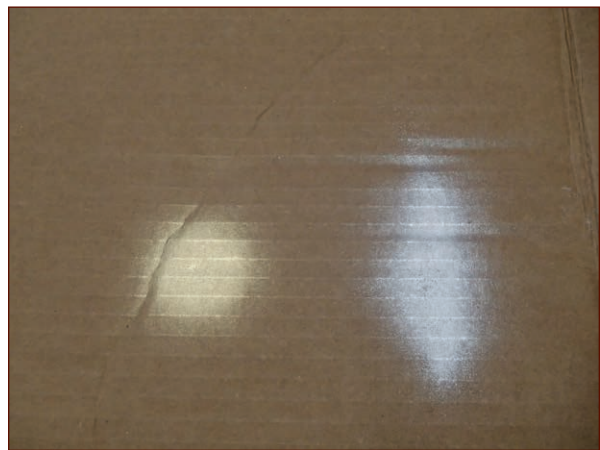
FIGURE 11-7: Spots of paint sprayed from two different cans showing their different spray patterns
