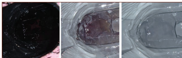
FIGURE 8-38: Going, going, gone. The casting resin changing color as it cures.
