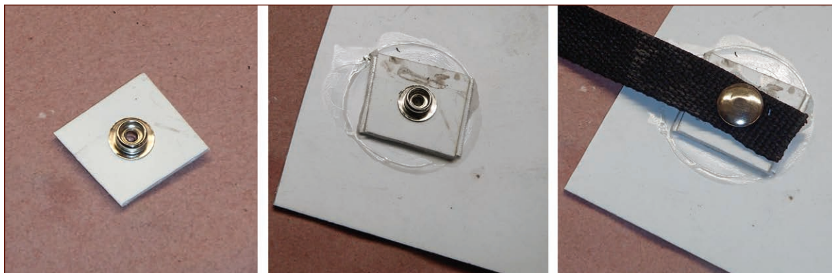
FIGURE 14-4: A good method of attaching snaps to vacformed armor without a visible attachment on the surface
