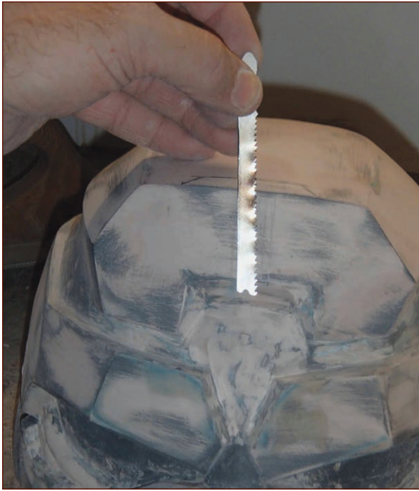
FIGURE 2-51: Using a loose jigsaw blade to make scribed lines groovy
