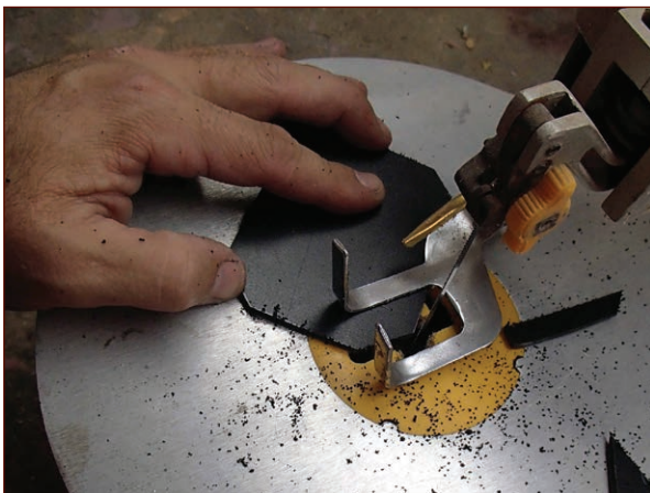
FIGURE 1-7: A scroll saw is ideal for making detailed cuts and even tightly curved shapes out of thin sheet stock.
