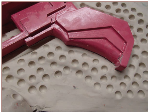
FIGURE 7-26: Any tiny clay remnants left on the prototype at this stage will become flaws on the castings later.
