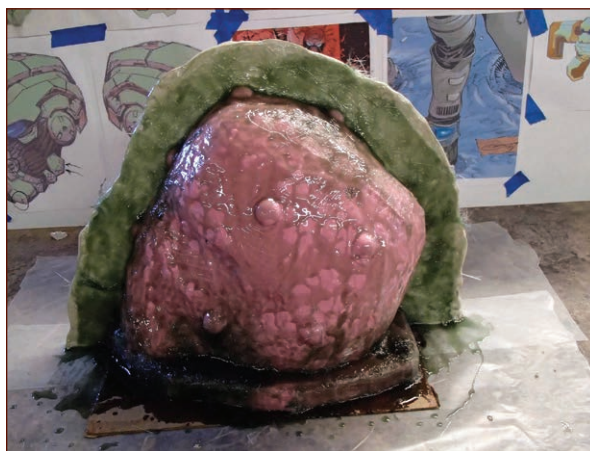
FIGURE 8-20: Putting fiberglass on the edges of the mold first ensures that nobody will forget to get them covered.
