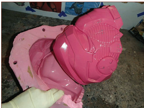
FIGURE 8-33: Removing the prototype from the rubber jacket
