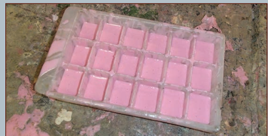
FIGURE 7-29: The half-filled ice cube tray makes good registration keys.
