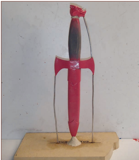
FIGURE 6-25: Vents added to allow bubbles to flow out of the mold
