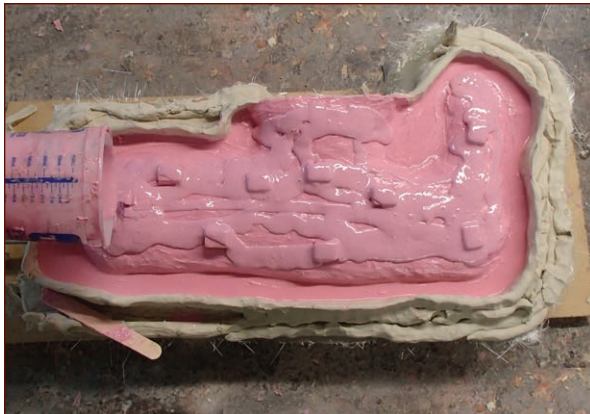
FIGURE 7-45: One more smooth coat of silicone
