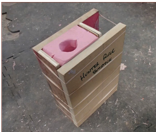
FIGURE 7-15: The mold box strapped together with rubber bands
