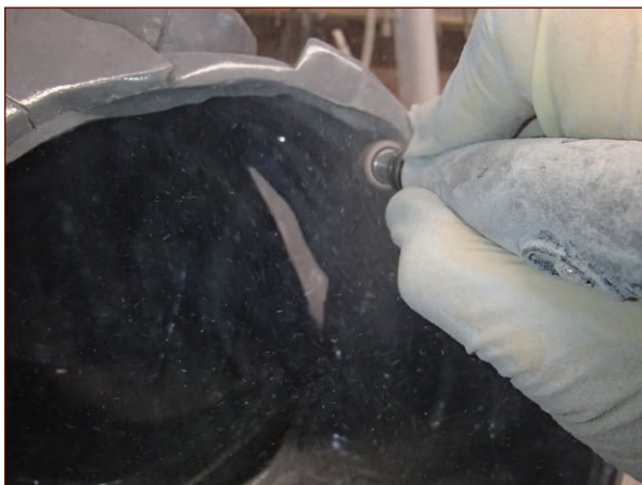
FIGURE 8-45: 80-grit sanding drum—because sometimes roughness is the best path to smoothness
