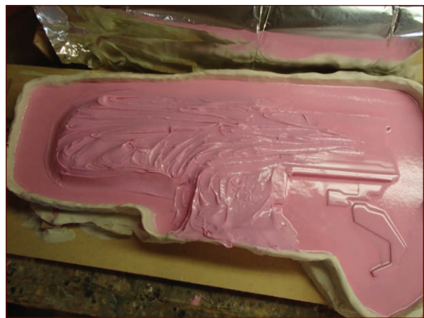
FIGURE 7-30: The rubber jacket halfway frosted with thickened silicone
