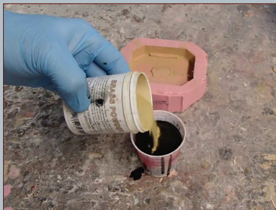
FIGURE 6-18: Casting resin with metal powder mixed in (brass in this case).
