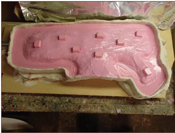
FIGURE 7-31: Registration keys added to the surface of the mold
