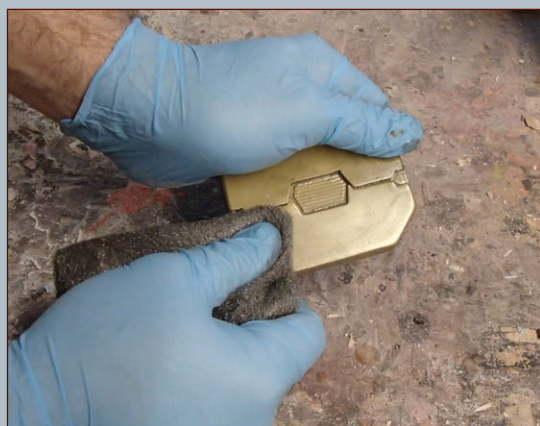
FIGURE 6-19: Buffing the surface to reveal the embedded metal powder
