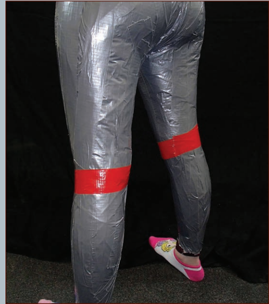
FIGURE 3-19: The red duct tape will make it easier to identify the knee joints on the finished dummy.
