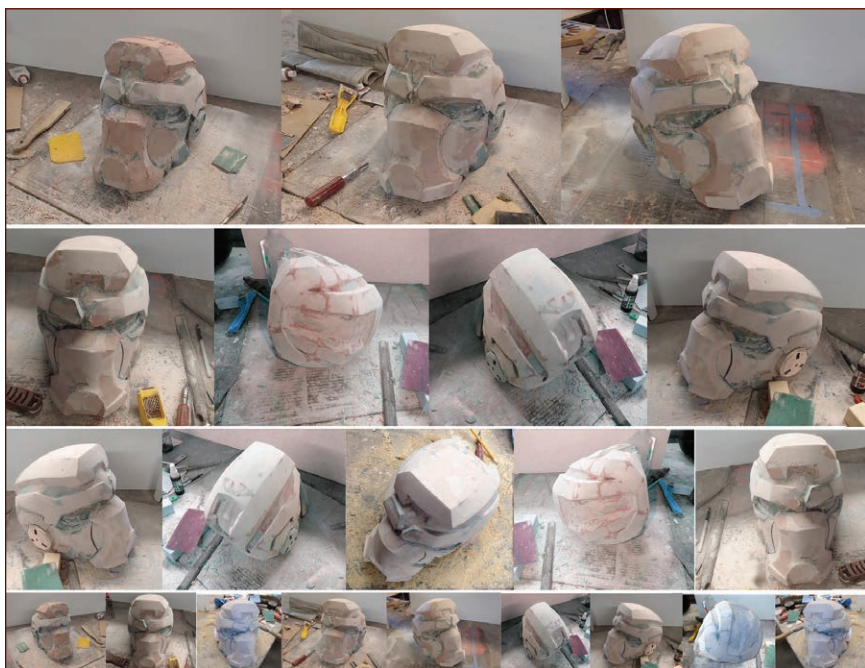
FIGURE 2-49: Filling and sanding and filling and sanding and filling and sanding and filling and sanding . . .
