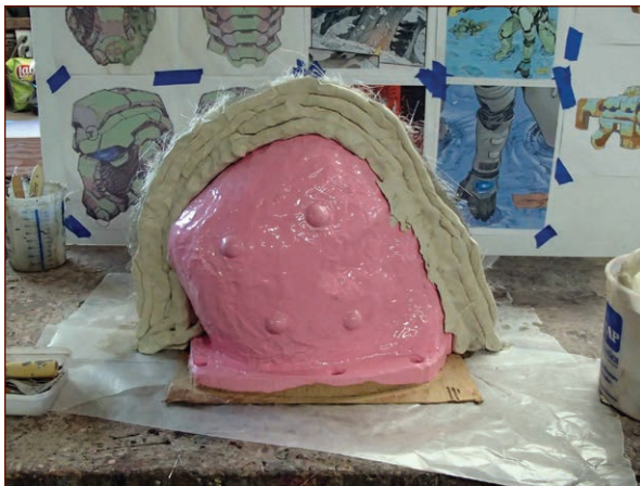
FIGURE 8-22: By the time you're looking at this angle, you're halfway done with the mother mold.
