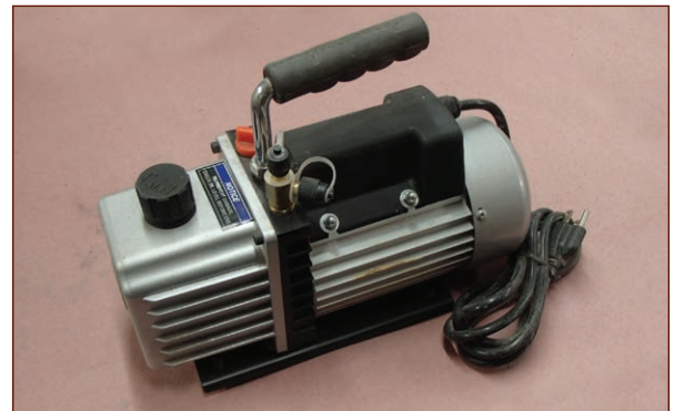
FIGURE 10-26: A small vacuum pump designed to service automotive air conditioning systems
