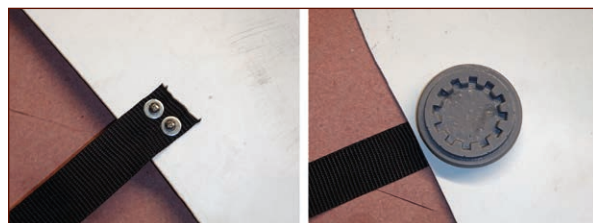
FIGURE 14-9: Small screws with washers (left) can be a great option for holding down straps when they can screw into a cast detail piece on the outside of thin plastic armor (right).
