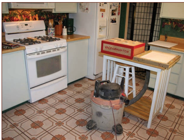
FIGURE 9-29: The forming platen plugged into the shop vacuum and positioned conveniently near the oven
