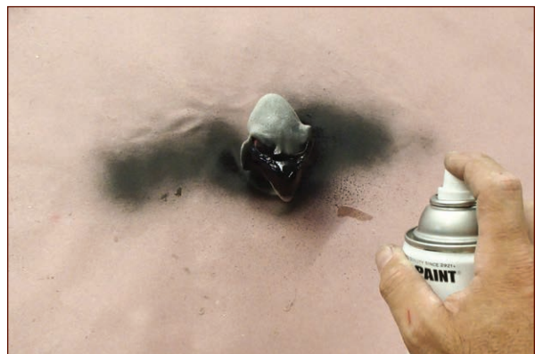
FIGURE 11-8: Start spraying before the can is aiming at the object and continue after sweeping past.
