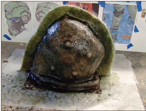
FIGURE 8-21: Fiberglass laid up across the rest of the mold
