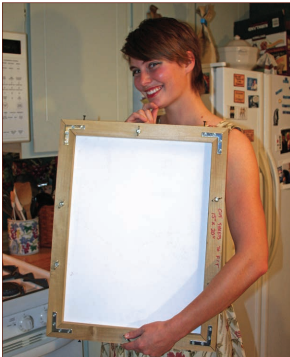
FIGURE 9-33: Clamping frame with plastic sandwiched inside
