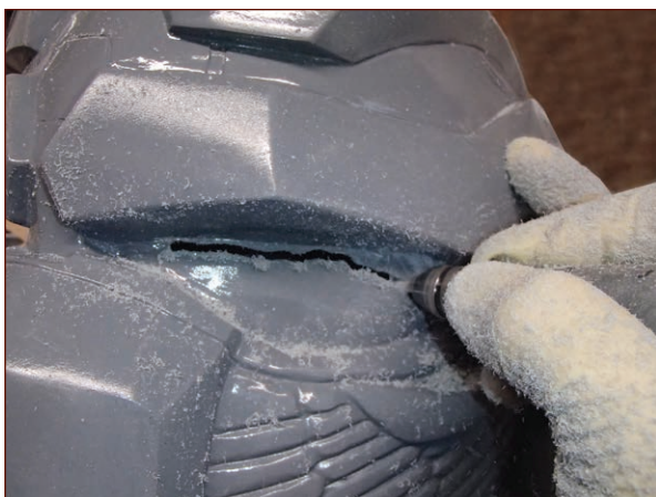
FIGURE 8-44: Rough trimming the eye holes, leaving material around the edges to be cleaned up later
