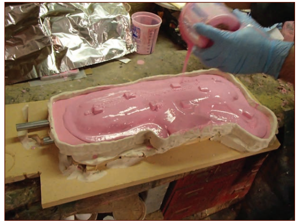
FIGURE 7-32: Smoother mold jacket
