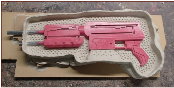
FIGURE 7-27: The clay bed, complete with a raised drip wall around the outside
