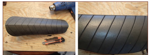
FIGURE 3-52: Making a seam line that's only skin deep
