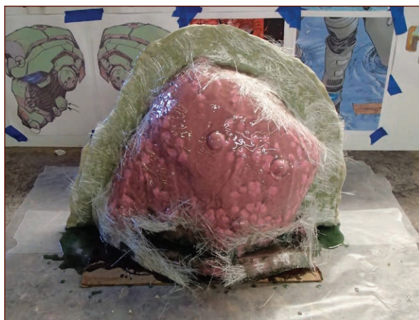
FIGURE 8-19: Fiberglass patches laid into the wet resin
