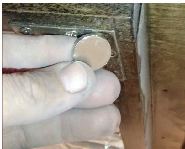
FIGURE 10-29: Magnets hold the clamping frame up to the heater.
