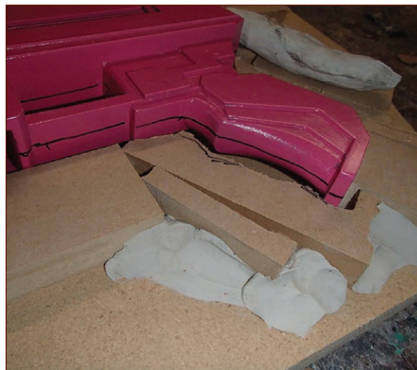
FIGURE 7-22: Blobs of clay to stick the blocks of scrap to the work surface
