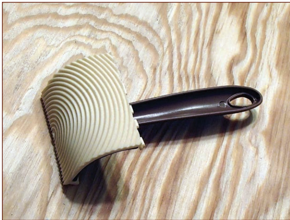
FIGURE 12-15: This is a graining tool.
