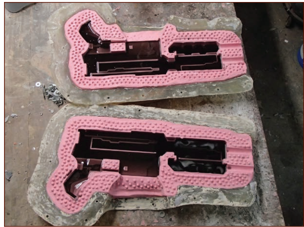
FIGURE 7-64: Coating the two halves separately puts gravity to work for you for a change.
