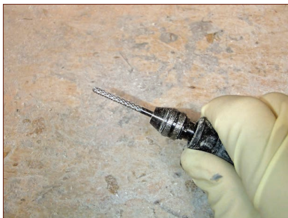
FIGURE 8-43: Designed for cutting ceramic tile, this bit does a great job of tearing through resin.
