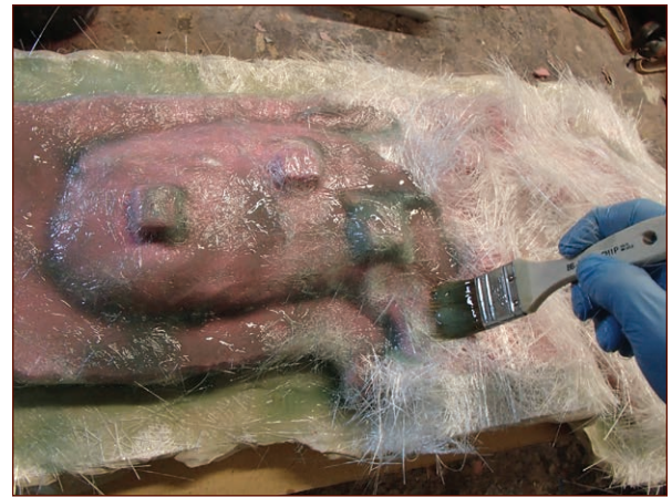
FIGURE 7-38: Brushing resin into (and bubbles out of) the fiberglass mat
