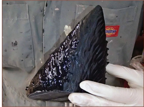
FIGURE 4-7: Using a specialized self-leveling resin to fill the build lines for the 3D printed ears
