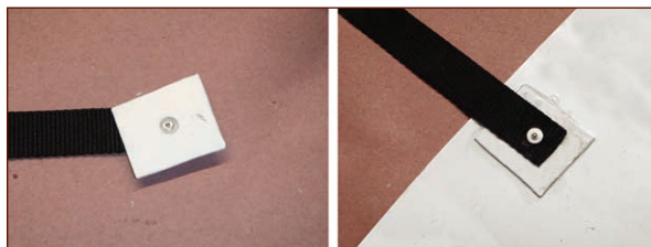
FIGURE 14-11: After riveting a piece of scrap plastic onto the end of a strap, that scrap can now be securely glued to the inside of the plastic armor using solvent adhesive.
