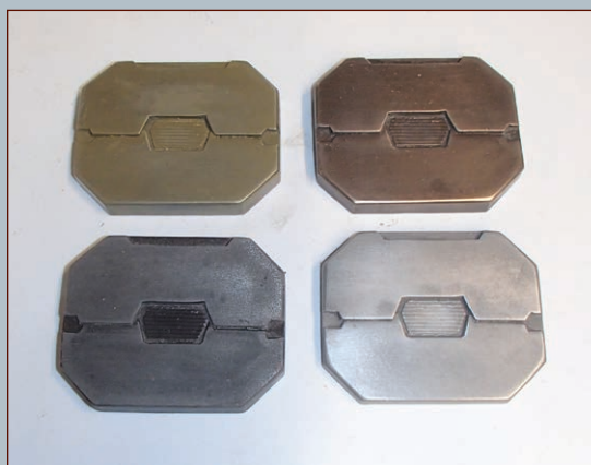
FIGURE 6-20: Hunter's belt buckle reproduced in faux brass, bronze, copper, steel, and aluminum.
