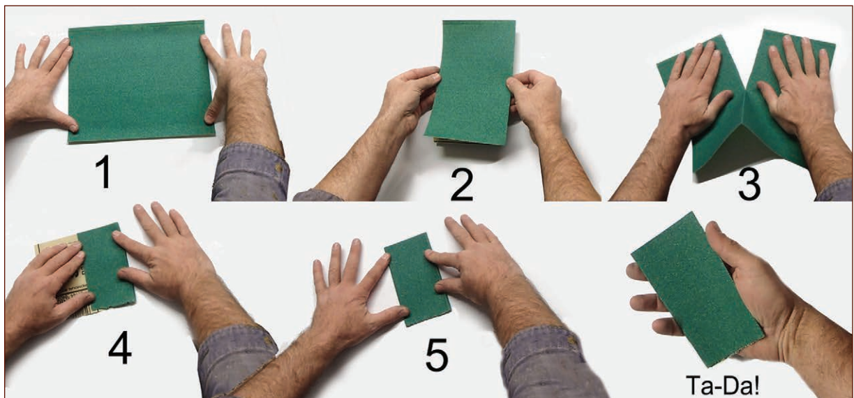
FIGURE P-4: This is the proper way to use sandpaper when hand sanding. Anyone who tells you otherwise is not your friend.
