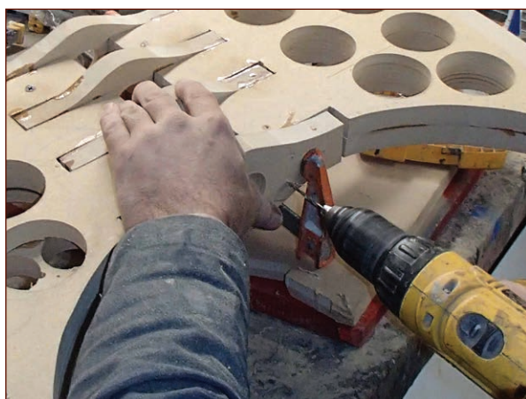
FIGURE 1-26: The pre-drilled hole will make it possible for the screw to effortlessly penetrate the MDF without splitting it apart.
