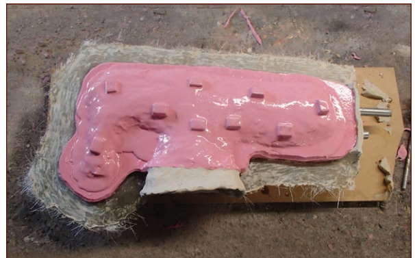
FIGURE 7-47: At this point, all of the clay has been removed except for the plug in the magazine well.
