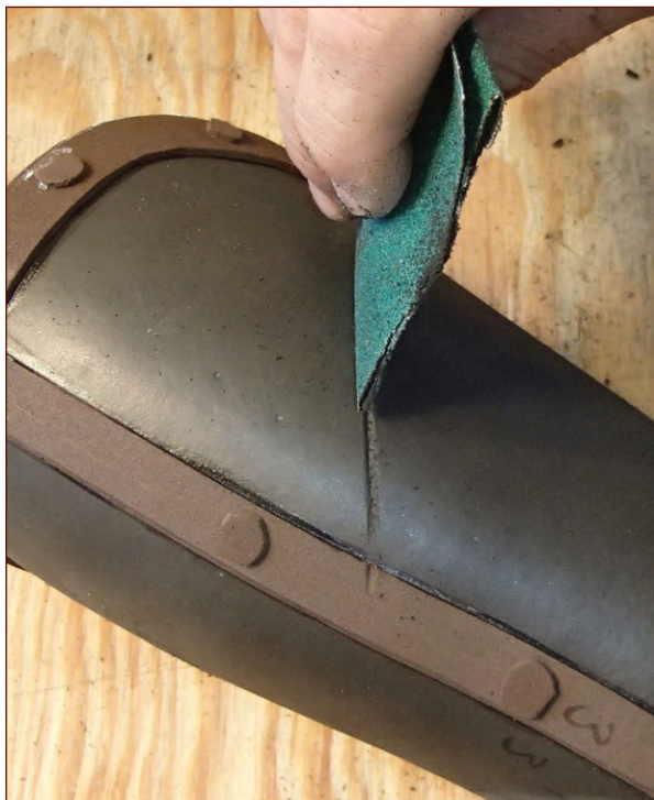
FIGURE 3-54: Scratches carved with a file and then heat-sealed
