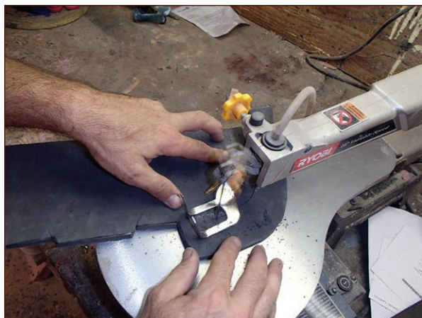
FIGURE 3-5: The scroll saw makes quick work of cutting foam.
