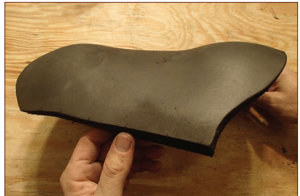
FIGURE 3-39: More heating, bending, and stretching to get the rounded shape for the elbow area
