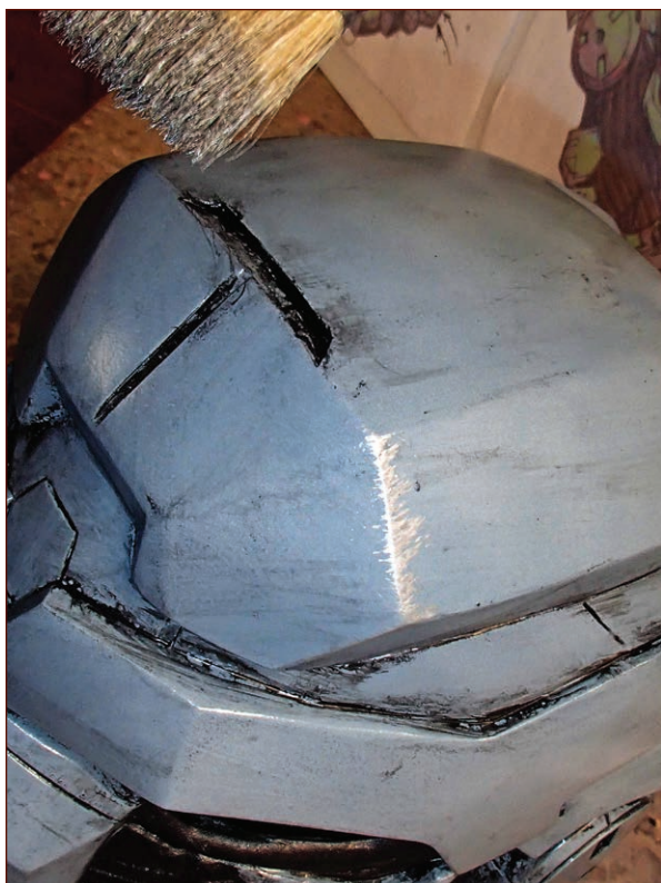
FIGURE 13-13: After dragging the nearly dry brush across the part, paint is only left on the raised edges.
