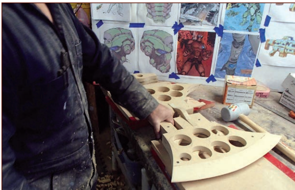
FIGURE 1-22: The blades propped up on some scraps of MDF so they'll stay straight
