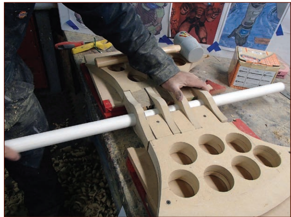
FIGURE 1-23: Keeping the handle in place makes sure that the holes will line up properly.
