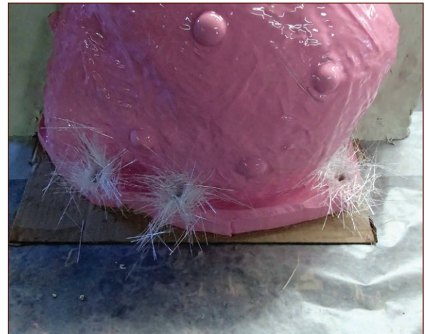
FIGURE 8-17: Peg holes loosely stuffed with fiberglass
