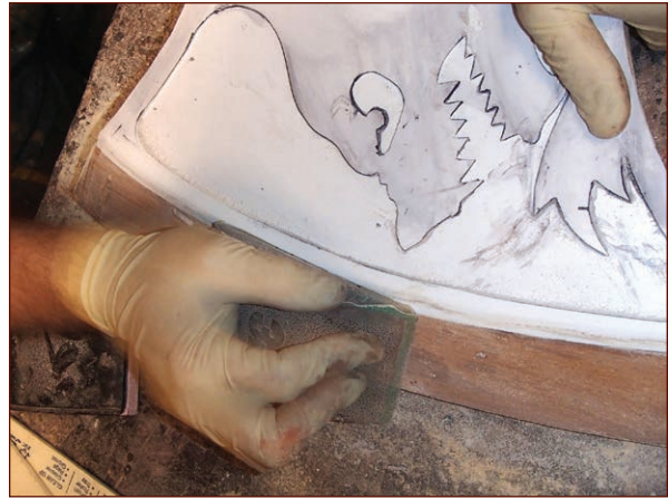
FIGURE 1-42: Smoothing the blade edge with a sanding block
