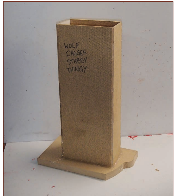
FIGURE 6-26: A better mold box, built to be reused if needed
