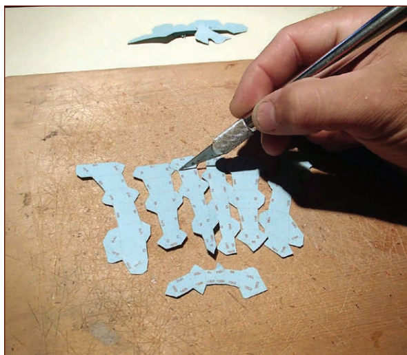
FIGURE 2-28: Gently scoring the fold lines with the tip of the knife
