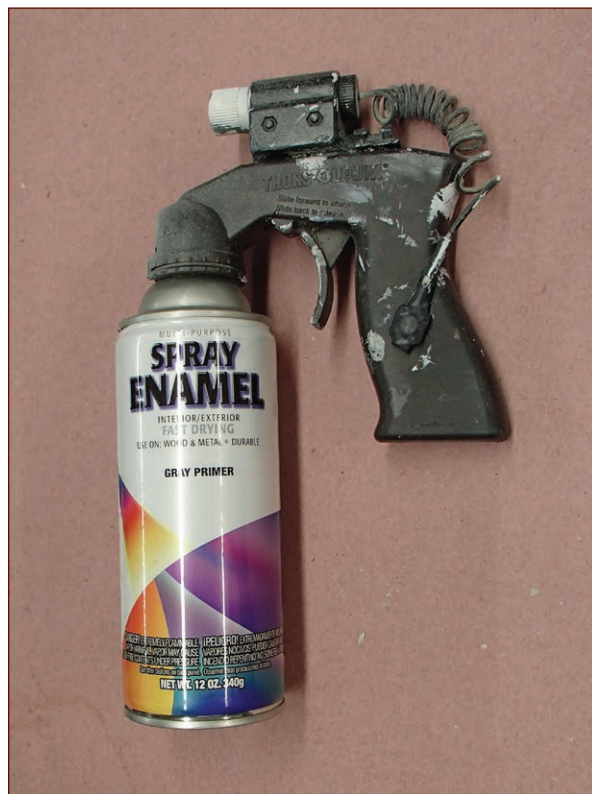
FIGURE 11-5: A typical spray can handle makes spraying easier on your hands. The laser sight was added later by the author. For accuracy.
