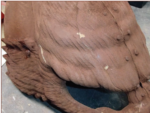
FIGURE 4-3: The MDF surface with a coat of red primer is still fuzzy.
