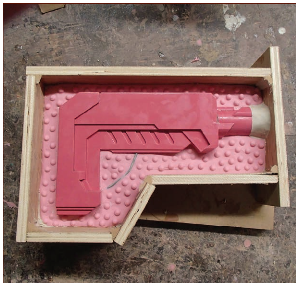
FIGURE 7-10: Bumpy silicone rubber
