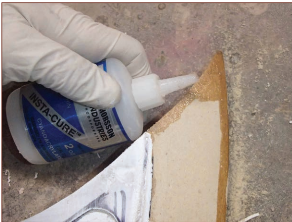
FIGURE 1-41: Soaking the edges of the blade with cyanoacrylate glue for strength
