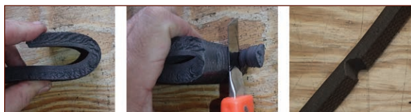
FIGURE 3-10: Cutting the inside out of what will become a rounded corner
