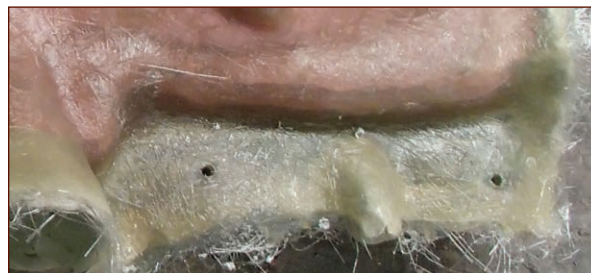
FIGURE 7-51: Bolt holes drilled in the flanges of the mother mold
