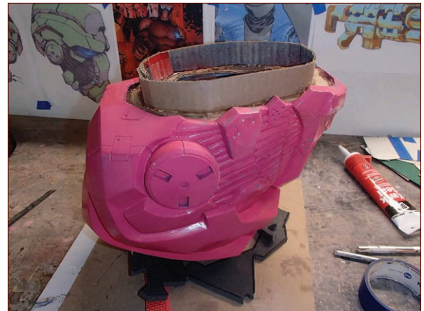
FIGURE 8-4: The cardboard wall that will later support the helmet
