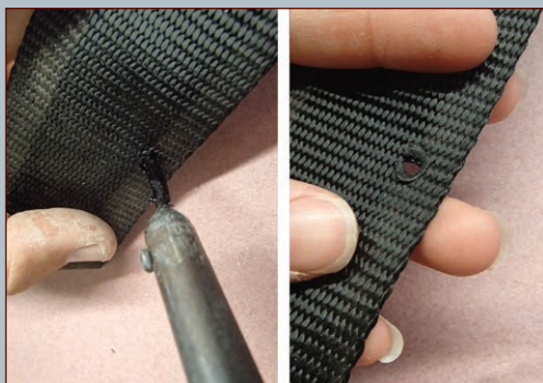
FIGURE 14-8: Using an old soldering iron to punch neatly finished holes through the webbing
