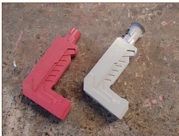
FIGURE 7-17: The first cast part pulled out of the mold
