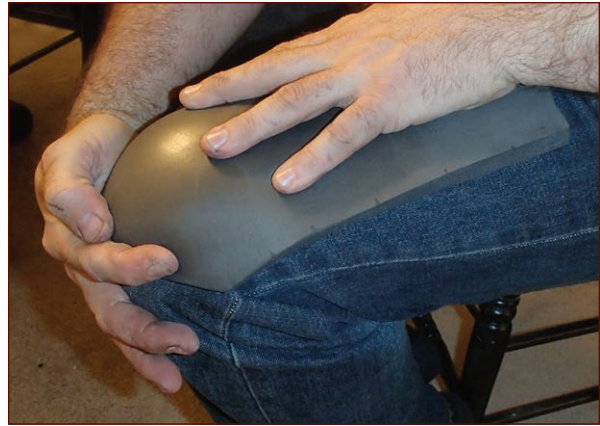
FIGURE 3-14: Pushing a bump into the heated foam by using a knee as a form
