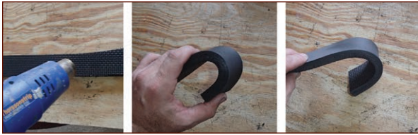
FIGURE 3-12: After you warm the strip with the heat gun and bend it by hand, it will keep its new shape when it cools.
