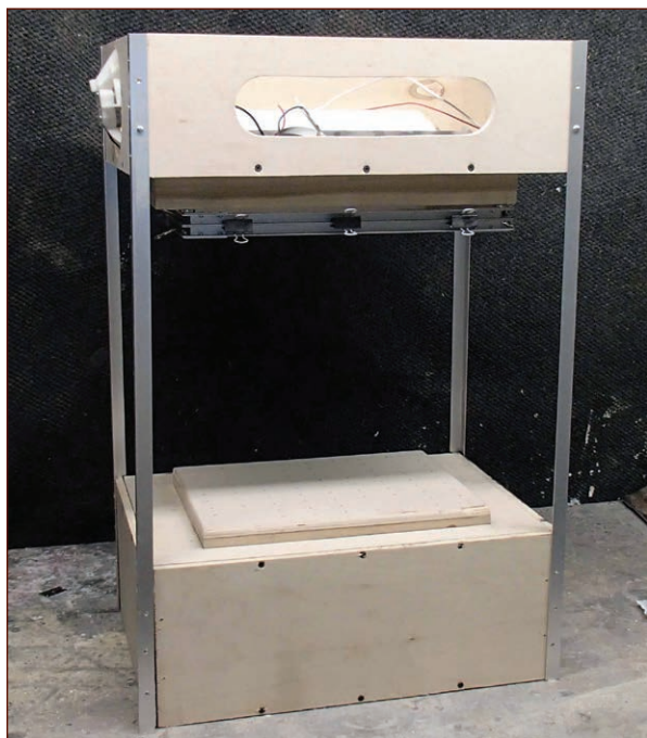
FIGURE 10-28: The assembled forming machine as a completely self-contained unit
