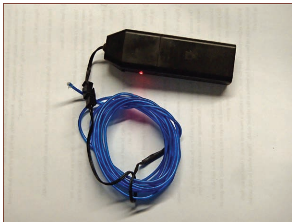
FIGURE 1-65: A neat little prepackaged EL wire system
