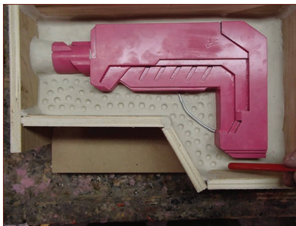
FIGURE 7-7: The finished clay bed, complete with dimples to form registration keys
