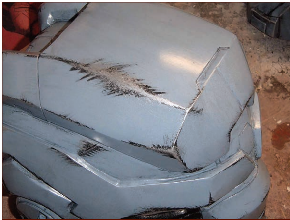
FIGURE 13-16: Shiny scratches and wear marks outlined with black for contrast
