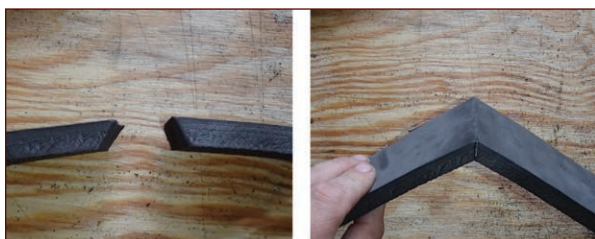
FIGURE 3-8: Viewed from end on, the angle-cut (or mitered ) pieces join together to create a corner.
