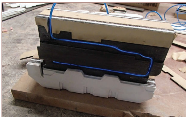
FIGURE 1-70: EL wire fitted into the grooves on the side of the forward section
