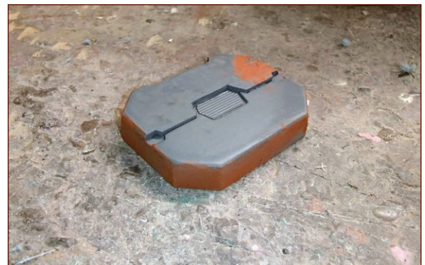
FIGURE 1-12: The edges coated with a smidgeon of spot putty
