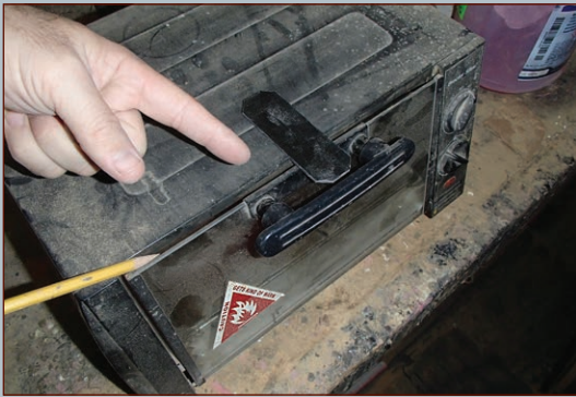
FIGURE 1-80: The gap in the door to the toaster oven concentrates released heat.
