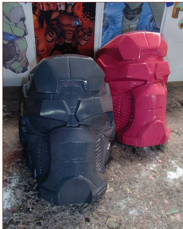
FIGURE 8-39: The strong, lightweight, rotocast copy next to the fragile, heavy, pink prototype
