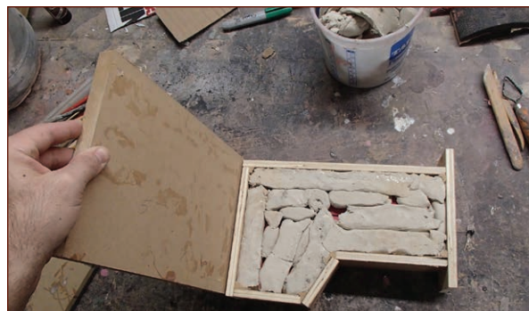
FIGURE 7-9: The mold box flipped over with its bottom removed
