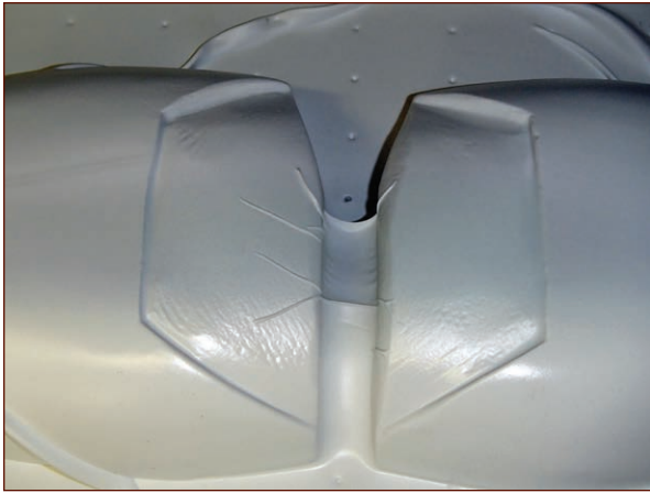
FIGURE 9-34: Webbing caused by having two forming bucks too close together
