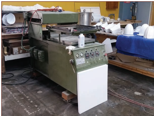
FIGURE 9-18: This old workhorse of an industrial vacuum former, now cranking out parts at 32Ten Studios, built an entire army of Stormtroopers back in the 1980s.
