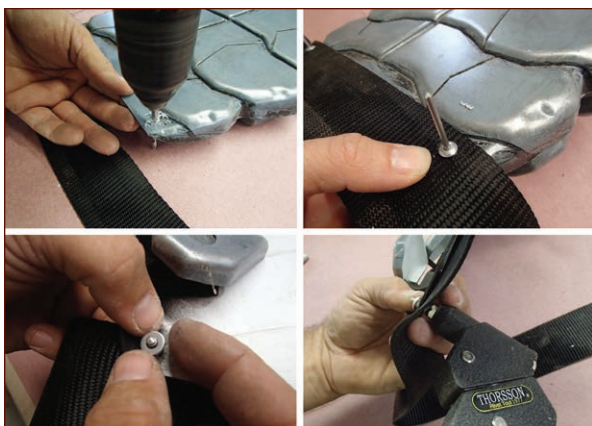
FIGURE 14-7: Installing a strap using a pop rivet and washer
