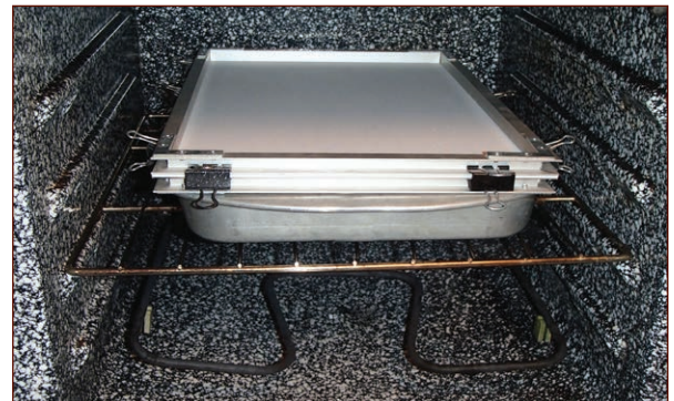
FIGURE 9-22: A small baking tray can be used to suspend the frame and keep the drooping, heated plastic sheet from sticking to the racks in the oven.
