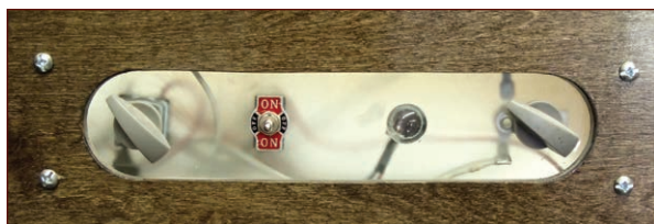
FIGURE 10-32: A piece of bottle green acrylic makes for a handsome mounting surface.
