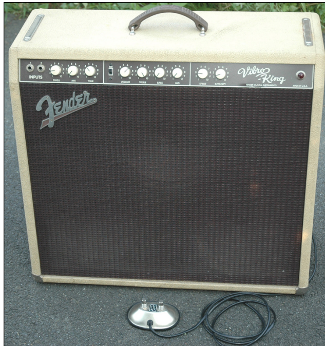
FIGURE 15-8: An amp with a footswitch- activated boost.
