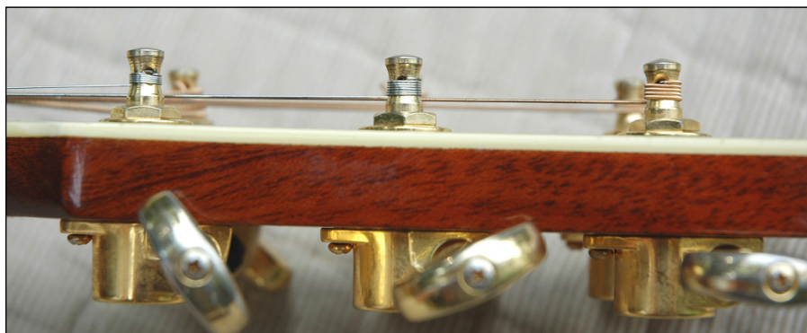
FIGURE 16-4: Coiling the string on the post.
