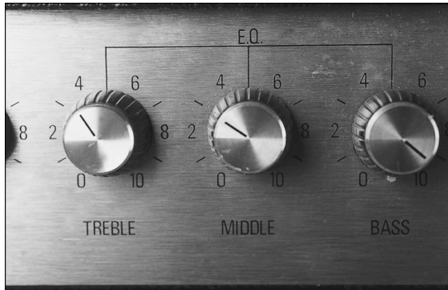
FIGURE 15-6: The tone section of an amp.
