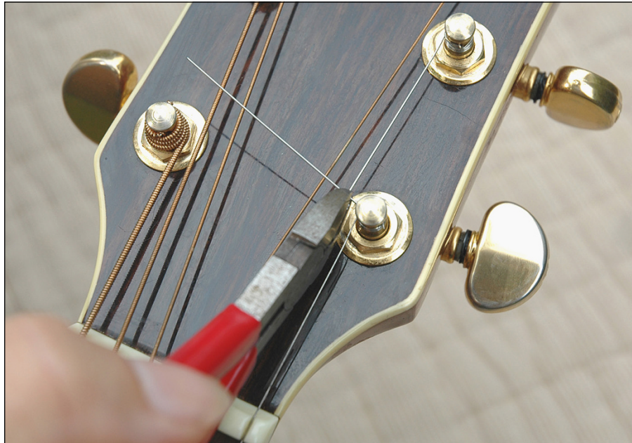
FIGURE 16-5: Clipping the string end close to the post.
