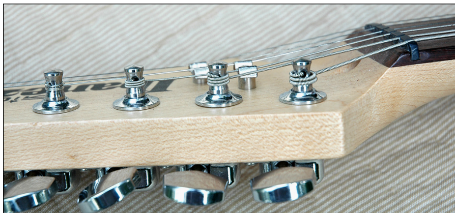
FIGURE 16-9: Coiling the string on the post.
