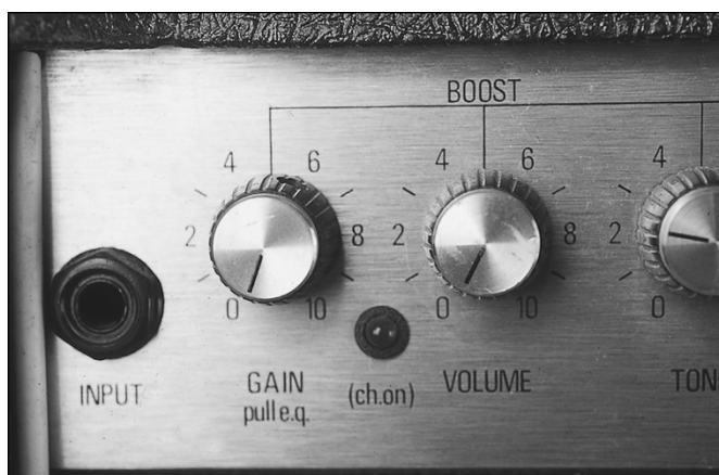
FIGURE 15-5: The preamp section of an amp.
