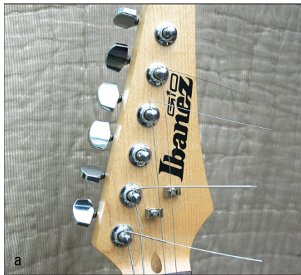
FIGURE 16-7: Kinking the string in the proper direction for inline and split tuners.
