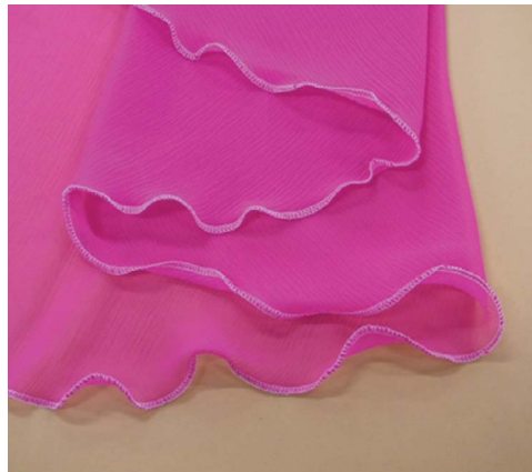
Figure 48 Rolled edge hem using 504 Three Thread Overedge.
