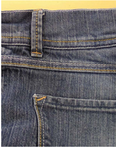
Figure 19 A condensed Zig Zag stitch called a Bar Tack is used to reinforce weak points on garments, such as the corners of a pocket mouth, and to attach belt loops.
