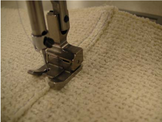
Figure 7 Used for stitching 5mm from the edge.
