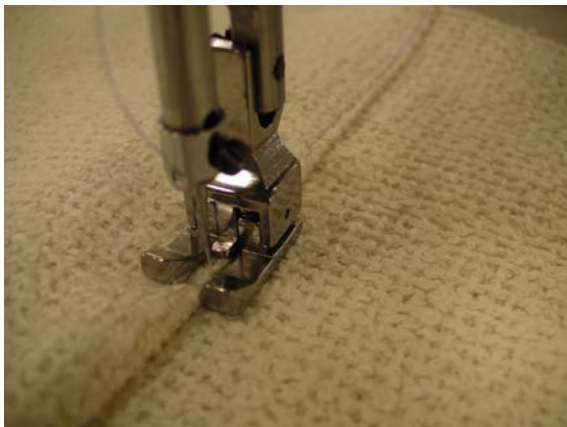
Figure 5 Used for stitching 1mm from the edge.
