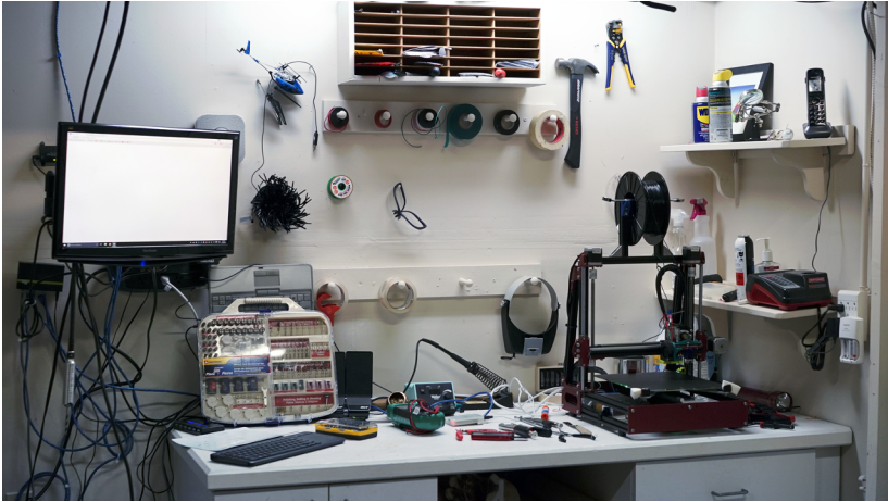
Figure 12-7. A loosely organized set of home workspace tools (multimeter, rotary tools, eye protection, soldering iron, and more)
