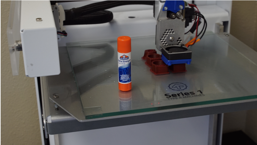
Figure 4-23. Consumer glue stick used to adhere prints to the build plate
