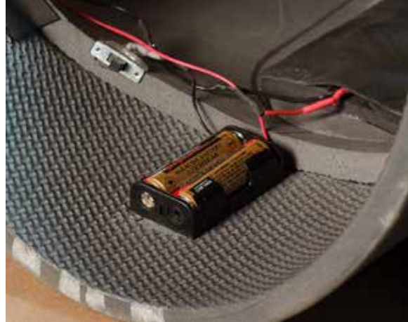
The switch and batteries for my Mass Effect armor hide behind my massive noggin.
