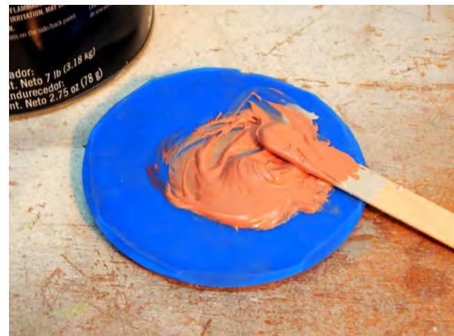
Using a mixing stick, mix the Filler with the Hardener until everything is a uniform color. Scrape the Mixing Board while mixing to ensure there's no unmixed Filler.
