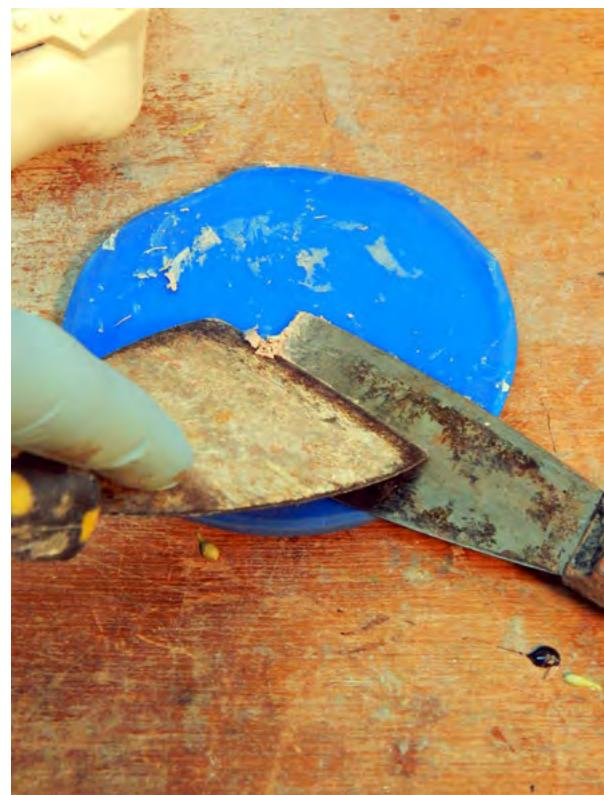
A putty knife or razor blade will easily shave the majority of the mostly-cured body filler off, and a few more quick passes to clean off any remainder will leave your tools ready for the next round of mixing and applying.
