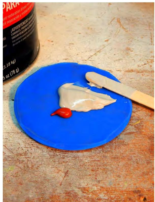
Next, squeeze an appropriate amount of Hardener onto your Mixing Board as well.
