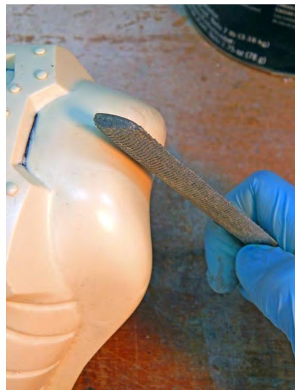
I like to use FLAT files to make CONVEX curves, and ROUND files to make CONCAVE curves.
