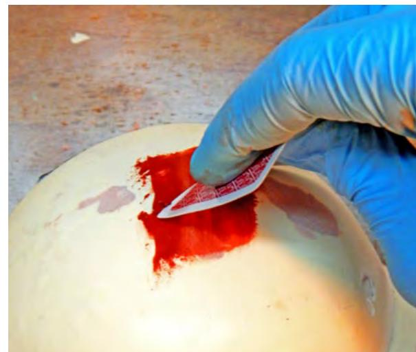
Skim a very thin layer of Spot Putty over the problems using a Spreader.
