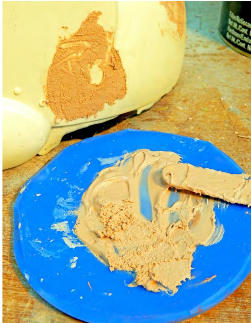
As it cures, body filler will start to heat up and get more stiff, moving from a smooth, frosting-like consistency to a slightly stiff, peanut butter-like one. It's still possible to shape it at this stage, though it's less sticky and pliable.
