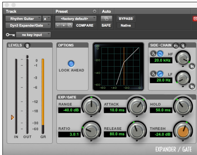
FIGURE 18-4: Use the gate plug-in to filter noise below a certain level.
