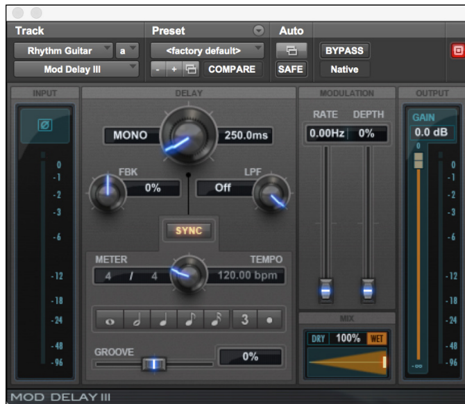
FIGURE 19-4: A Delay plug-in allows you to create various echoes.
