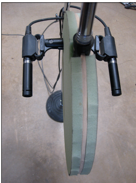
FIGURE 7-8: A Jecklin disk can make stereo recording easy and capture an awesome, natural sound.
