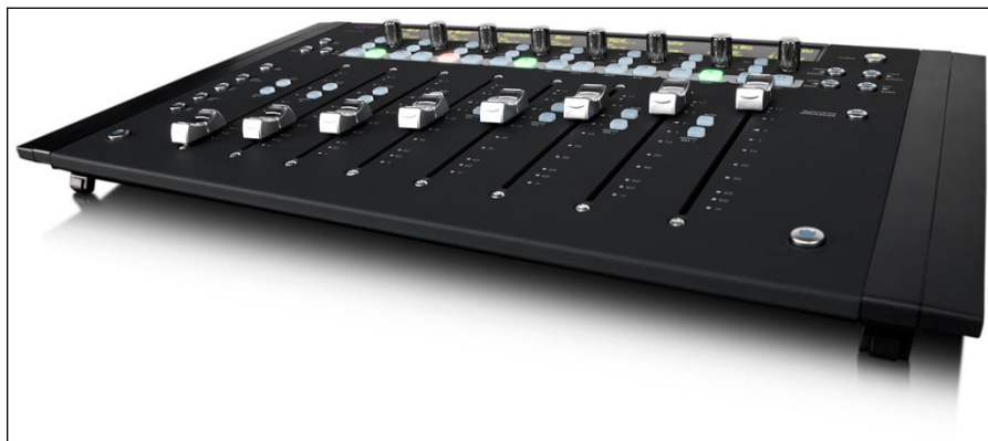
FIGURE 16-1: Mixing with Avid's Artist Mix control surface lets you use your hands to control the mix.
