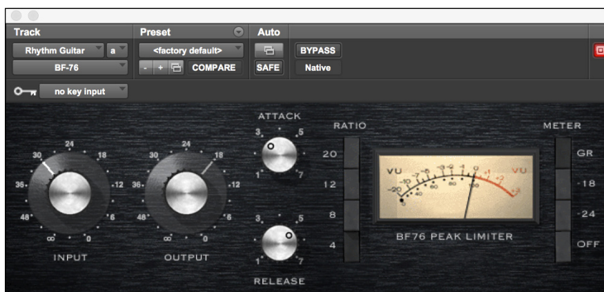
FIGURE 18-3: The peak limiter plug-in limits the maximum level of the signal passing through it.
