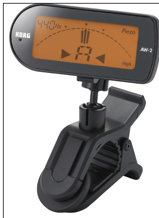
FIGURE 2-16: An electronic tuner uses visual feedback to help you get in tune.
